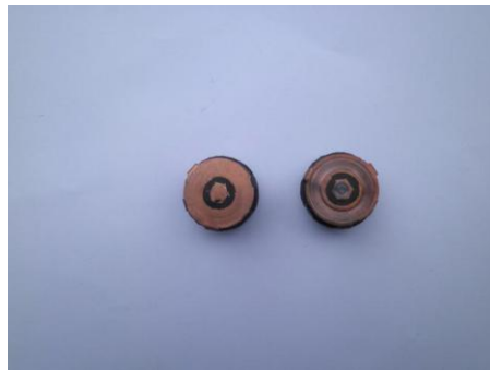
The new slip ring alongside the old one.
