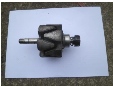
Rotor now free of the DE bracket.
