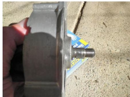
The rotor refitted to the DE bracket. The wider distance is positioned prior to fitting the key.
